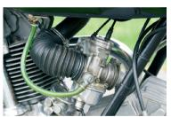
Dell-Orto PHF 30A carburettors were fitted towards the end of 1973, but the pleated plastic air intakes remained.
