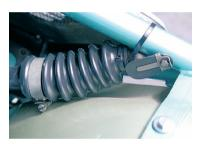
The crankcase breather for the 750 SS (and some 1974 750 Sports), included a bellows and flapper valve.
