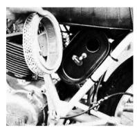
The engine breather valve exited into the rear air filter box.
