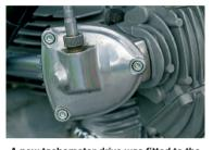
A new tachometer drive was fitted to the front cylinder head during 1973. This was for Veglia or Smiths instruments.
