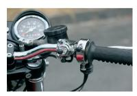
The right Aprilia indicator switch mounted on a specific triangular plate.
