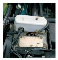
With the Dellorto carburettors the regulator moved to a plate under the seat next to the fuse box.
