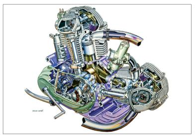
A cutaway of the 750 GT engine.
